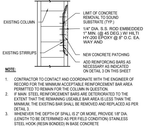
AT 9" O.C. WITH 2" EMBEDMENT. THE HORIZONTAL LEG OF THE HOOK SHALL BE 2" LONG MINIMUM.
